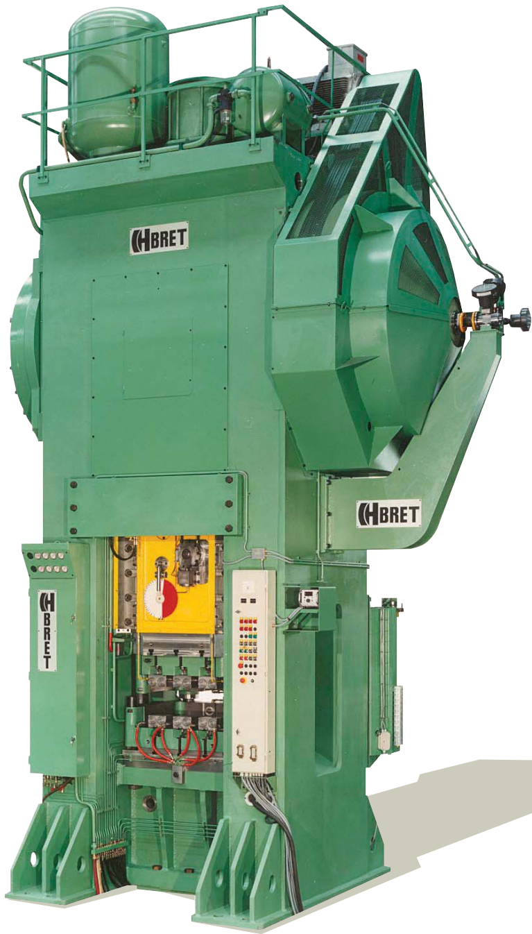
Presse de forge 1 600 tonnes. 1 600-ton forging and die stamping press.
