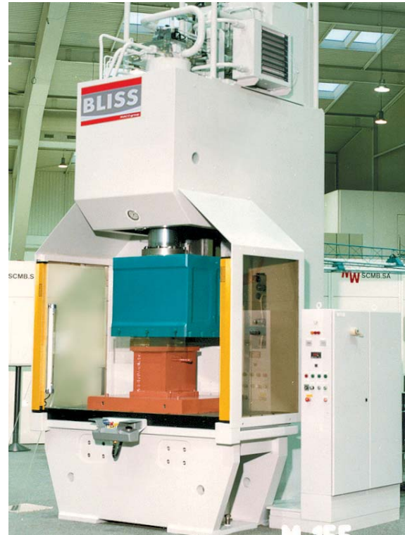
Presse type PHCm160, table de 1000 x 800 mm. PHCm160 press, 1000 x 800 bolster.
